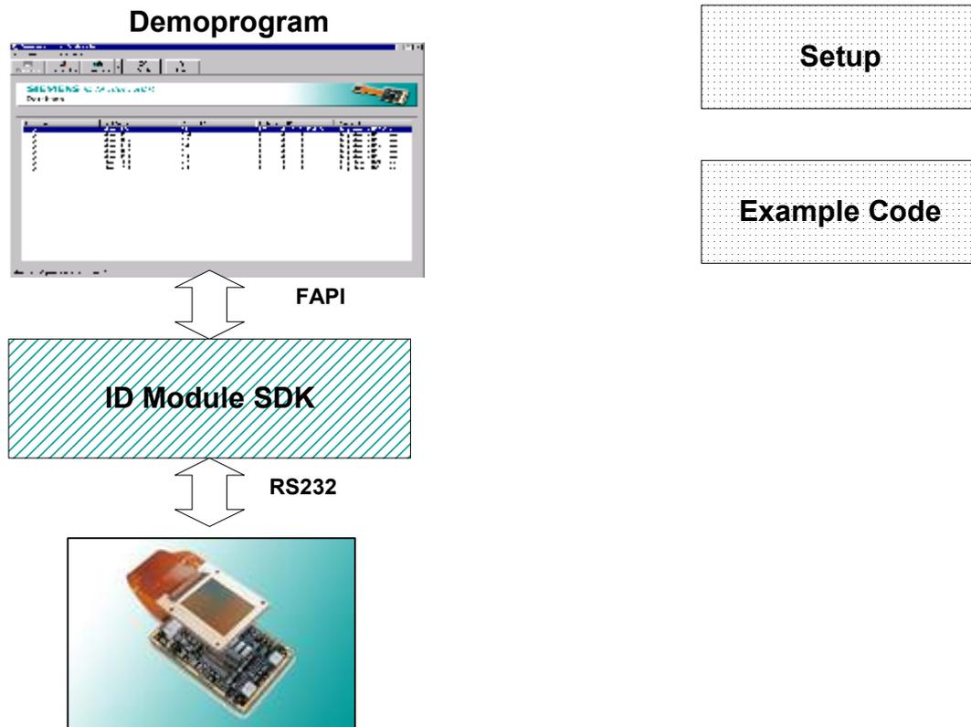
**Figure 2-2: Block Level View of ID Module SDK**
