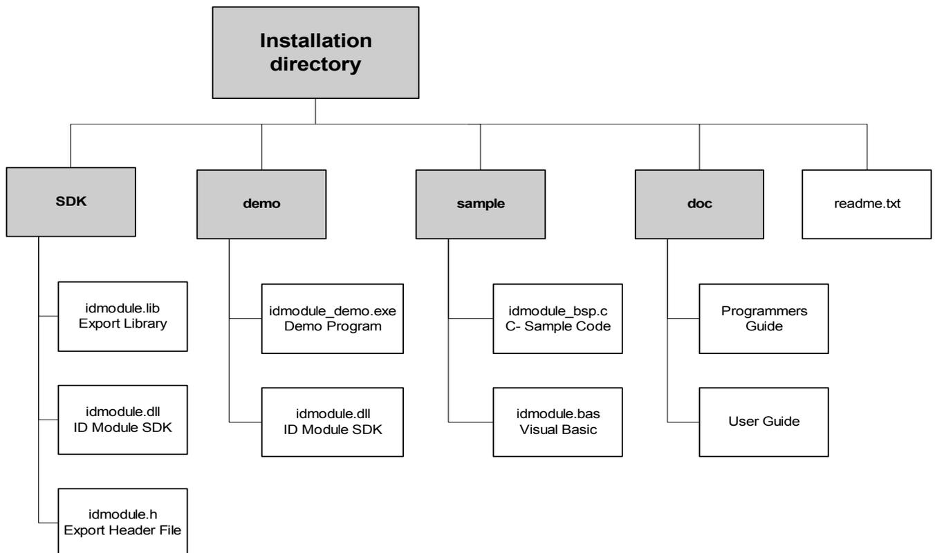
**Figure 5-1: Structure of ID Module SDK Software Package installation**
